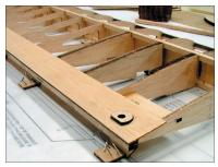
Glue on the laser cut 1/4" trailing edge, make sure the laser cut hinge slots are facing aft and the root and tip are oriented correctly. The root has a larger slot cut for the aileron linkage installation. Sand the trailing edge and false trailing edge to the contour of the wing and then add the 1/16" balsa trailing edge sheeting.
