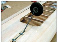
Du-Bro steel landing gear straps are used to retain the landing gear leg.
