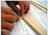
Glue a strip of 3/8" triangle stock along the top edge of both fuselage sides on the labeled side. Be sure to align the stock with the recessed edge as shown. Also add triangle stock to the bottom fuselage edge for and aft of the wing opening. Note the markings on the fuselage, they indicate where to stop the triangle stock.
