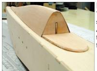
Trim and sand the top deck to shape as shown and then add the cockpit floor. Angle sand the cockpit floor as shown to accept the windshield later. The basic fuselage structure is now complete.
