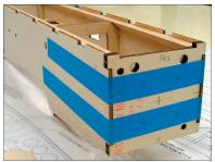
Use Epoxy to install the firewall onto the fuselage. Use masking tape to assure good contact between all parts. Note that 1-1/2° of right thrust is built into the firewall.
