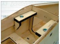
Epoxy the wing mount plate braces in place as shown. Then flip the assembly over and add a 1-1/4" piece of triangle stock gusset to the top of each wing mount plate. You can access this through the holes in the fuselage top.
