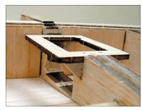
Glue the aileron servo tray into position and brace it with some triangle stock gussets as shown. NOTE: Not shown here, install the two sheet support rib sections to the top of the servo tray along both sides of the servo opening. These supports look like the drawing below.
