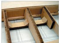
Assemble the 1/4" ply main gear mount and the 1/8" ply main gear mount retainer plate. The end of the slot in the retainer plate aligns with the hole in the main gear plate. Install this assembly into the notches provided in WGB, W3-B and W-4-B. The end of the assembly with the hole in it should be pointing toward the
