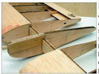
Assembly sequence of the wing joiner. Apply Epoxy in the spar box, on the spar, to the joiner and ribs forward of the spar and to the joiner and ribs at least 1" behind the servo knockout. Make sure both wing halves align at the trailing edge and secure in that position with pins until cured. Long strips of masking
