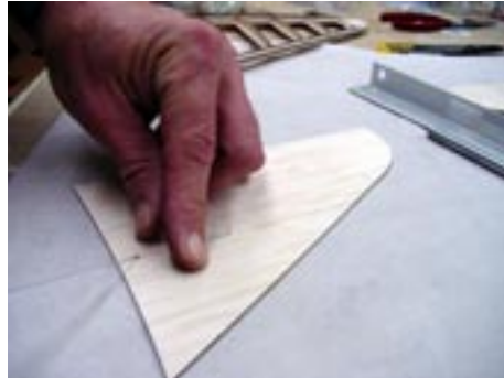
Here the laser cut fin sheeting is being assembled over parchment paper with thin CA.
