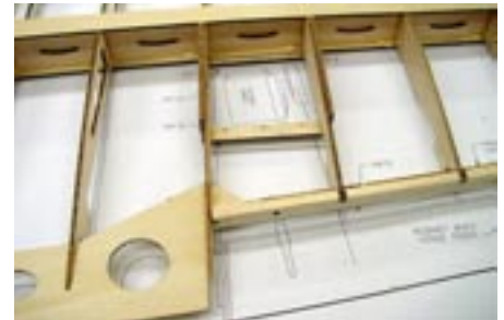
Aileron bay trailing edge (ABTE) keys into all wing ribs. Note that in this photo the aileron servo mount rails have already been installed. You will get to those later.
