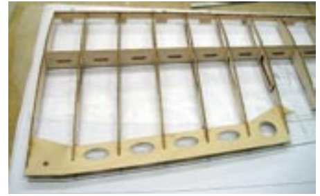
The 1/16" ply trailing edge keys into all wing ribs. It must tip into rib W-7, then slide forward into remaining ribs.
