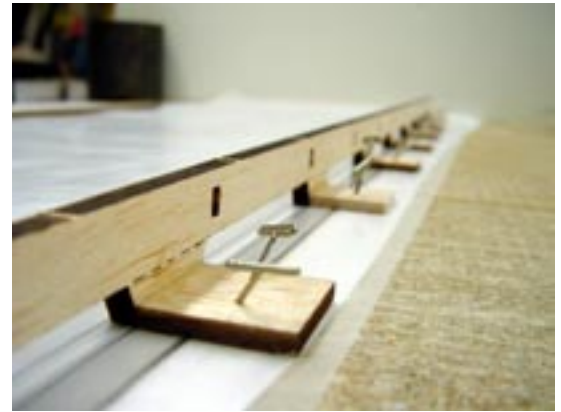
Pin tabs are used to secure FLE to the building board.
