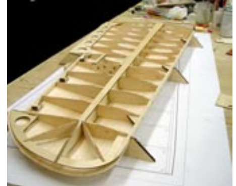
Wing assembly suspended on the rib jigs at W2, W7 and W12. These jigs will support the wing assembly while the bottom sheeting is being installed.
