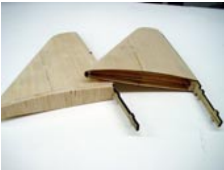
After assembly add two layers of scrap 1/16" balsa to the bottom of the assembly as shown in this before and after example.
