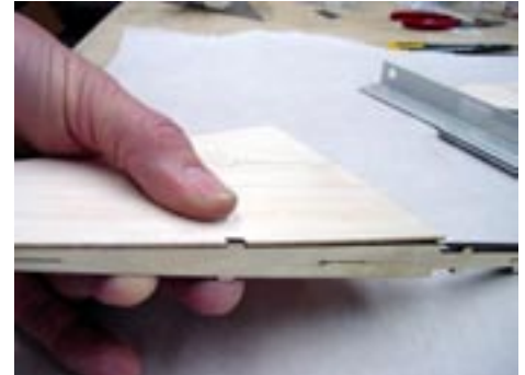
Here the fin sheeting is being installed. Note the tab on the rudder post will provide exact positioning.
