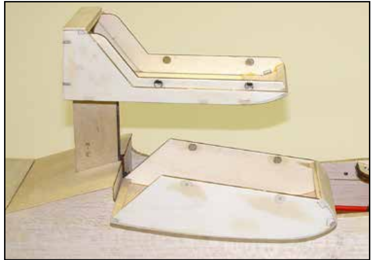
The completed power pod installed on the pylon with the water resistant hatch removed. This pod can hold a 6 oz. tank for glow power or the motor controller and battery for electric power.
