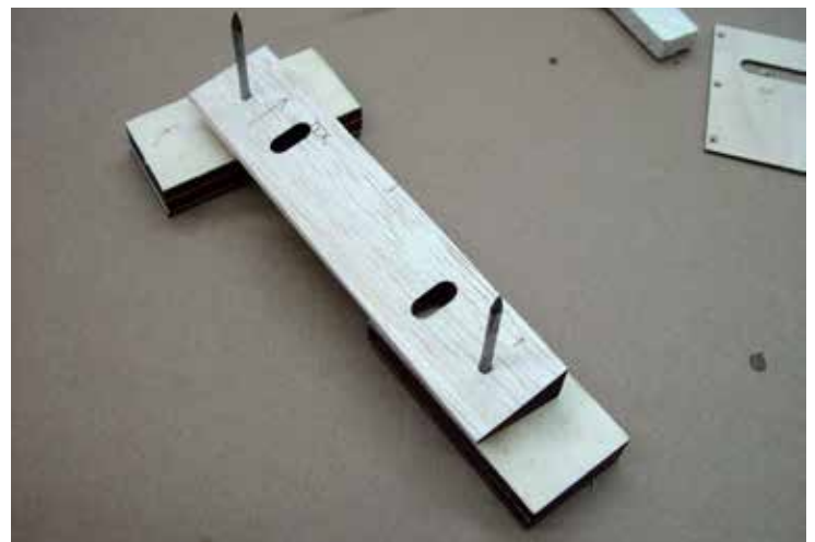
Laminate the two trailing edge extensions (TEX) using the pin registration system, keep the labeled sides out.
