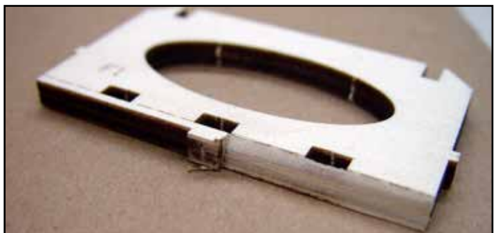
Here only half of the bottom of F1 has been beveled to the dashed line to accommodate the curved bottom sheeting. Leave the tab until after the sheeting has been attached.
