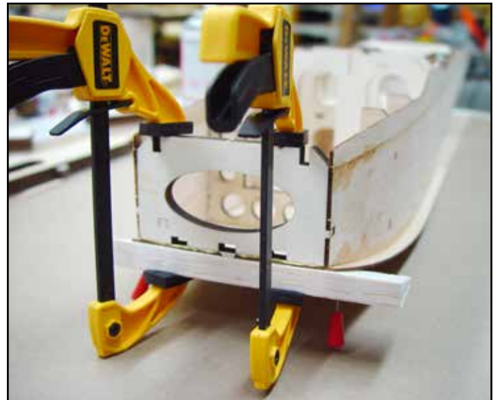
Installing the fuselage bottom, a piece of scrap balsa is beveled as required to provide the clamps a flat surface to grip.
