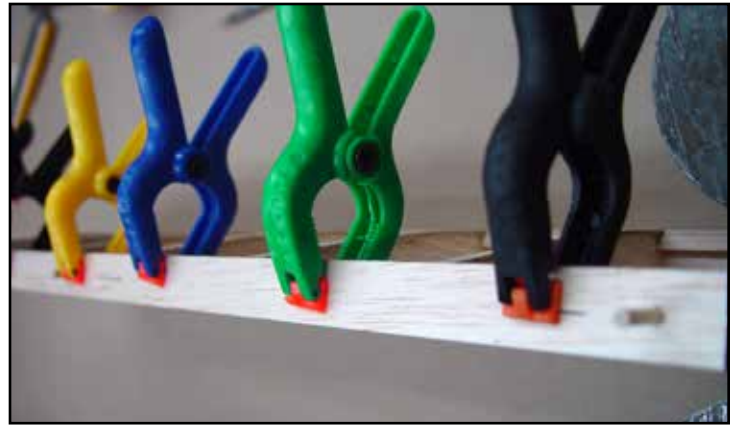
Dowels are used to precisely position the trailing edge and clamps secure it until the glue sets.
