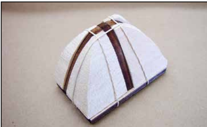
ABOVE: The four nose cone blocks have been marked and all excess material will be cut away prior to assembling the nose block. LEFT: The nose block has been assembled and rubber bands are used to hold the assembly together until the glue sets.
