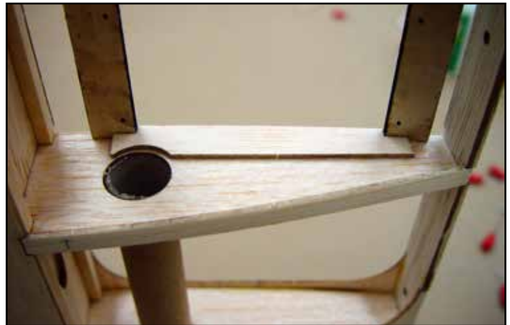
W5-A and W6-A are installed as shown above, they will provide a ledge that the servo mount will rest on.
