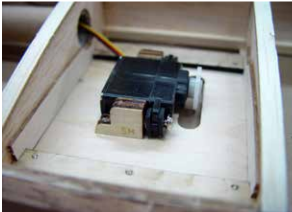
Aileron servo showing the servo mount installation. Use plenty of CA on the ply mounts.
