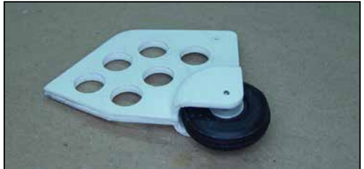
The completed tail gear assembly ready for land operation.
