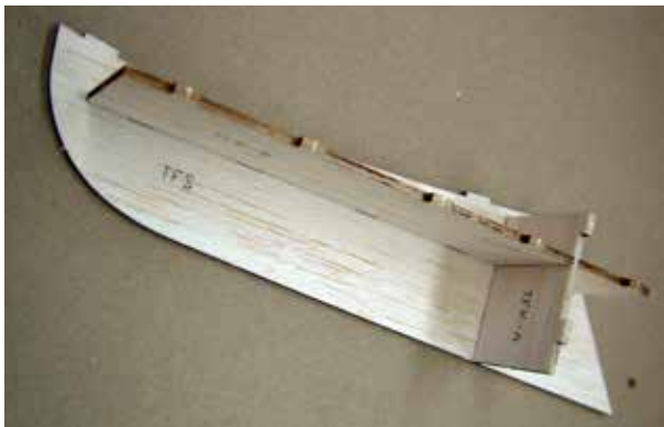
ABOVE: Pontoon construction begins with the assembly of TFK-A and TFK-B, then the sides are installed. RIGHT: The pontoon assembly ready for sheeting. Tabs will position it on the bottom wing sheeting.
