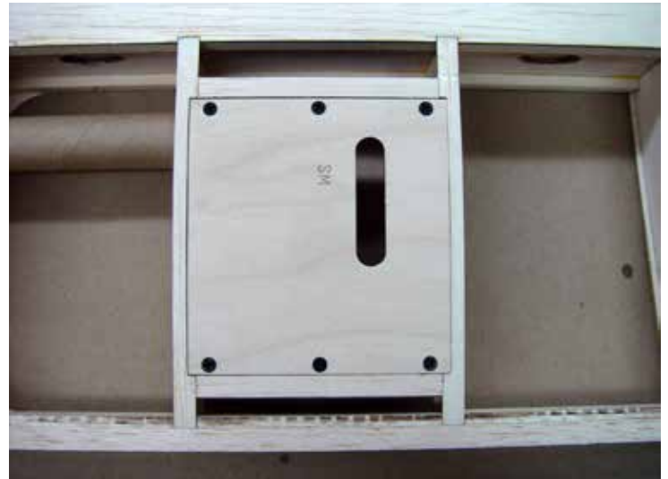
The servo mounting plate should fit snugly to help waterproof the servo and wing assembly.
