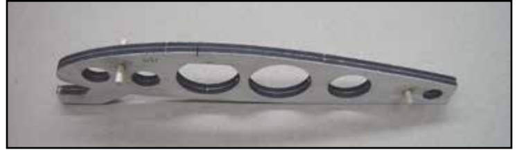
The wing hook assembly with dowels installed, ready to join the wing halves.
