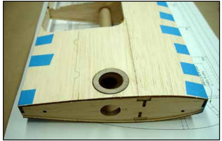
Here the bottom leading edge and center section sheeting have been installed and tape is used to secure the sheeting until the aliphatic resin has set.
