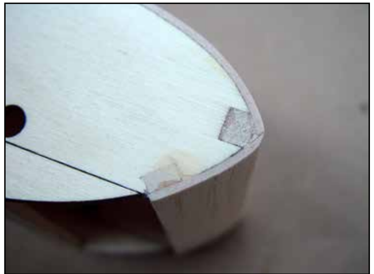
The hatch top sheeting is assembled above, note the dash cut opening at the front of the assembly will be opened later on the electric version only.
