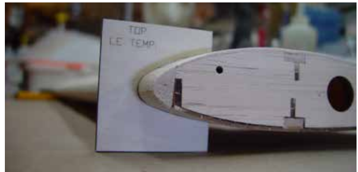
Use the leading edge template to help in shaping the leading edge.
