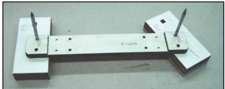
MGP-S parts are glued to the MGP-A assembly.
