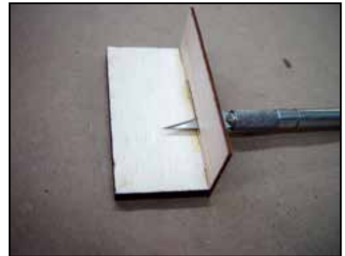
The rudder is laminated from three sections, the ply center section has cutouts for the hinges and the kick-up water rudder is mounted to the bottom.
