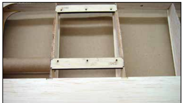
The ply servo mounts are installed between W5 and W6.
