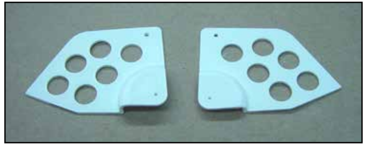
Plastic tail gear mount halves will replace the water rudder for land operation.
