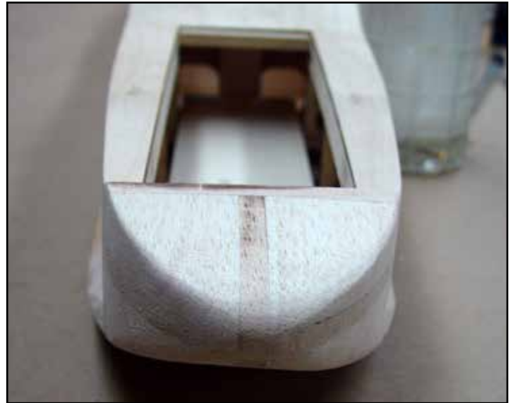
This method of producing the nose cone makes it easy to maintain symmetry and reduces much of the carving needed.
