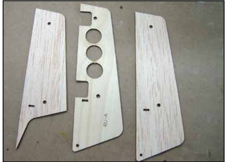
The rudder is laminated from three sections, the ply center section has cutouts for the hinges and the kick-up water rudder is mounted to the bottom.
