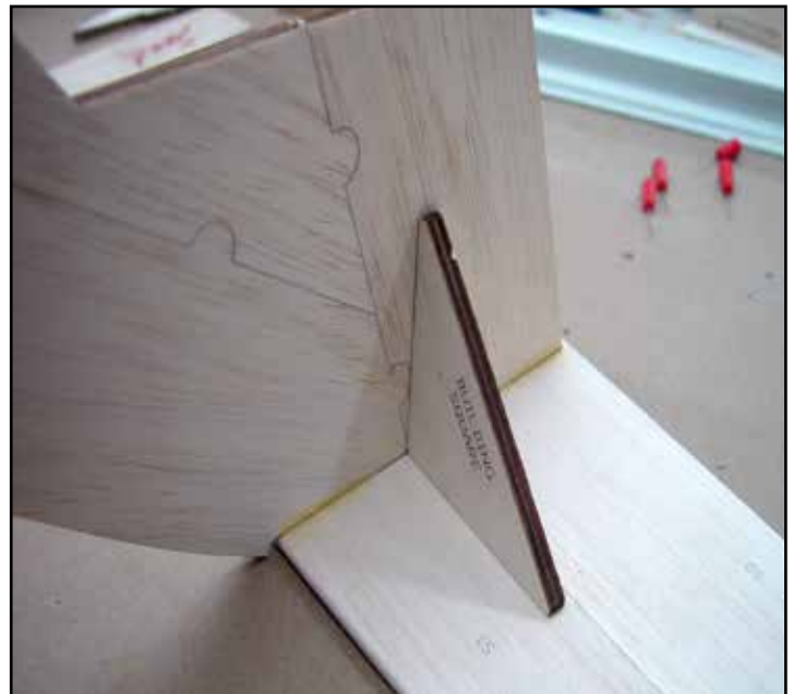
Use the building square to insure that the vertical fin is installed perfectly square to the stabilizer. Reinforce the joint with 1/4" triangle stock.
