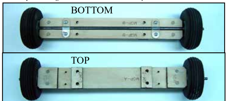
Top and bottom view of completed mains gear.
