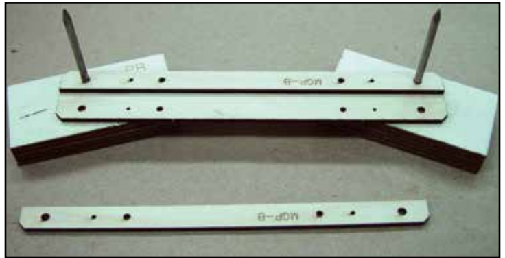
Registration pins are used to install MGP-A and MGP-B with the labeled side of MPG-A down.
