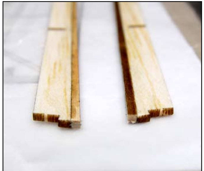
ABOVE: A 1/16" square basswood spar has been laminated to the bottom of the sheer webs in preparation for assembling the wing inboard section.
