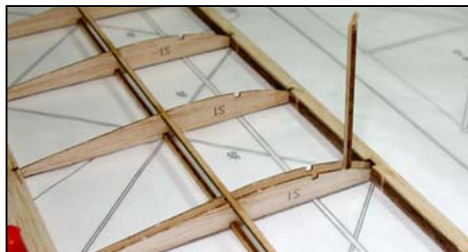
ABOVE: Use a scrap piece of 1/16" stock when installing the two center ribs to insure proper spacing for the stabilizer hook which will be installed after covering.
