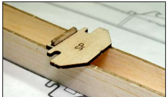
BELOW: The stabilizer platform is installed onto BH-6 and the fuselage top.
