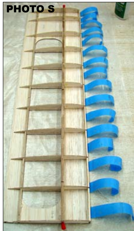
Photo S: In preparation for installing the top wing sheeting, masking tape has been applied to the bottom leading edge of the wing.
