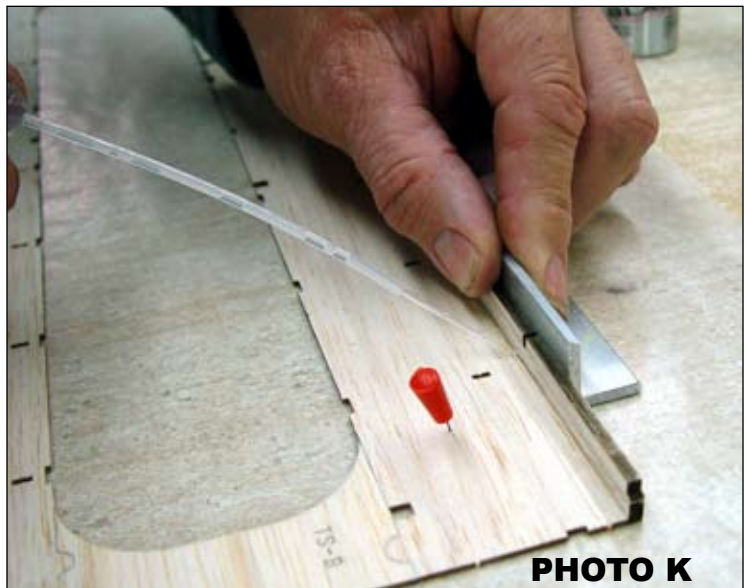
A short length of aluminum angle is used to align FLE with the leading edge of LES-B while thin CA is applied with a pipette applicator.
