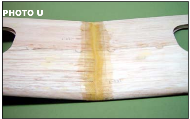
A strip of fiberglass cloth over the center joint will add considerable strength to the wing. This one was brushed with thinned Epoxy resin but you can also use thin CA to attach it.
