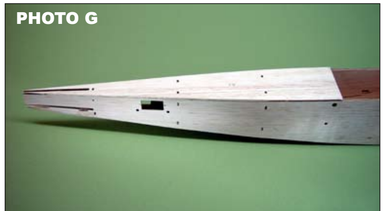
The aft top sheeting (F8) is installed. To insure a perfectly straight fuselage, make sure the tabs in F4, F5 and F6 are fully engaged in the slots in F8. Install F8, turn the fuselage over and apply CA through the open bottom of the fuselage.
