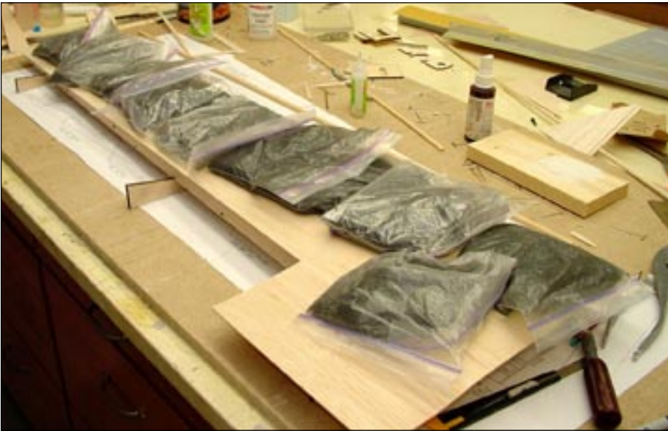
Here the bottom skin is curing with lead shot bags applying pressure. The wing is supported on three balsa jigs that conform to the airfoil.
