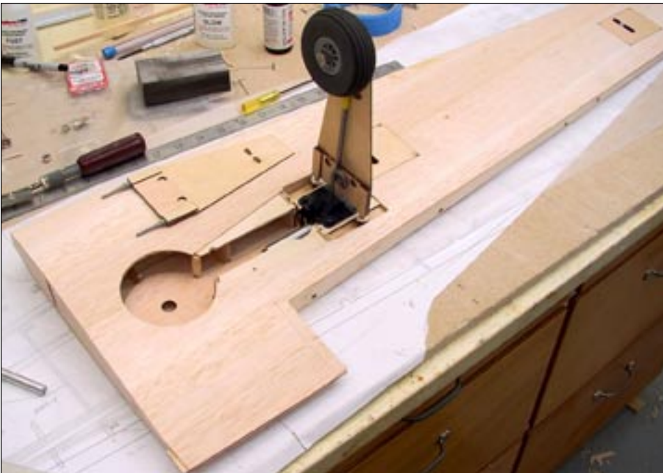
Here the gear opening has been cut, the gear and gear door temporarily installed. The gear door is used as a template to remove the wing sheeting for a snug fit. The gear well lining will be installed after the wing halves are joined and the belly pan constructed. The other gear door assembly is laying on the wing just above the well opening.
