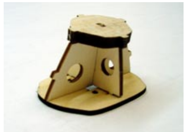
This sub assembly of F-1 and F-2 simplifies the installation of these components. It also assures the correct rake angle of F-2 to accommodate the nose gear mount.
