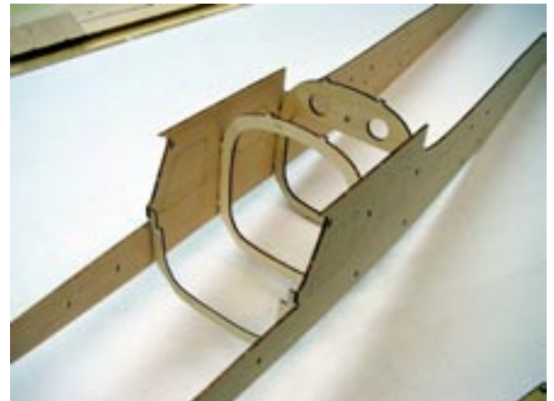
Construction of the fuselage begins by gluing only a 1" area of the formers between the tabs to the fuselage sides. This will allow forming and gluing the fuselage sides to the formers after all formers are in place.
