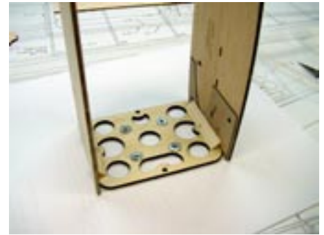
Nacelle sides, firewall and nacelle doublers are assembled at 90° to each other as shown. Install the #4-40 blind nuts before gluing firewall in place.
