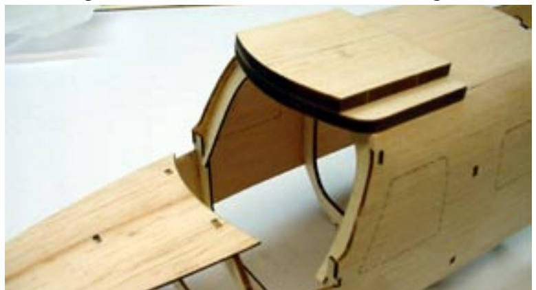
After installing FCR-A and FCR-B, shaping of the forward cabin section can now begin.
