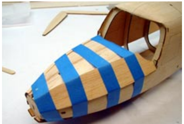
After installing the cabin roof sections a guide line has been drawn and the forward section is tapered from that point to the cabin opening.
