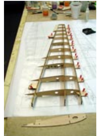
Wing rib W-1 is installed after the optional cable tunnel tubes are installed.
