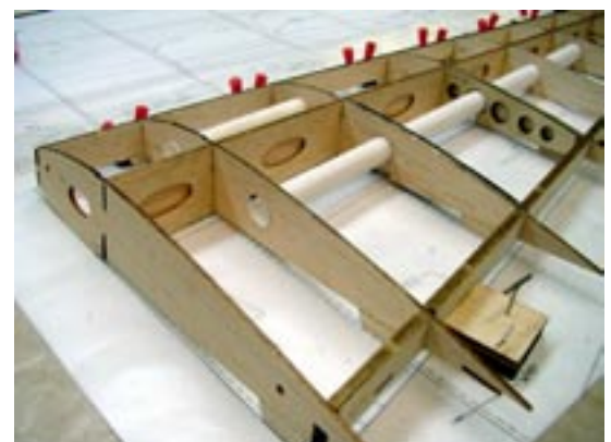
Note that the sheer web and the leading and trailing edge set the correct dihedral angle of W-1. The 1/8" holes in W-1 will align with dowels in WJ to assure perfect alignment of both wing panels.
