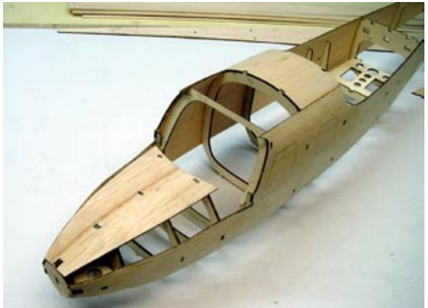
After all formers are glued, the top fore deck and cabin top are installed. The fuselage sides will now be planed flush with the top of F-5A in preparation for the installation of FCR-A and FCR-B.
