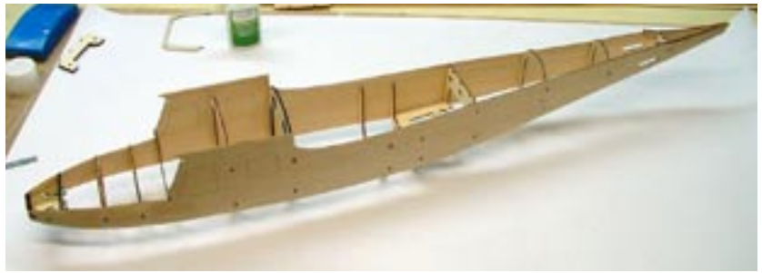
All formers installed, now the fuselage sides can be formed to the contour of the formers and gluing completed.
